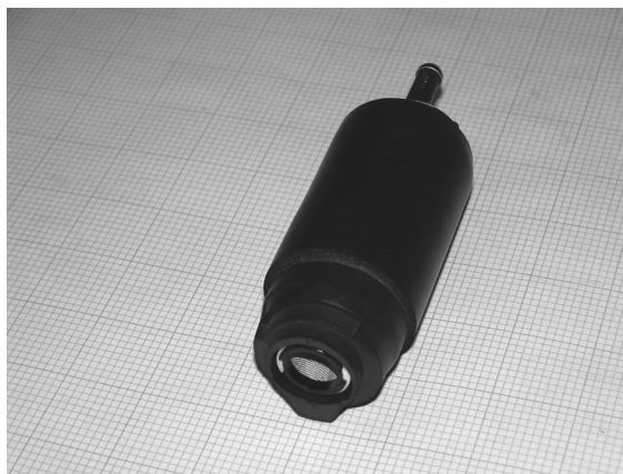
— FIGURE 19 — NOTE ORIENTATION OF BOOTY TIP TO PUMP DISCHARGE
